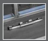
All Wagon HD models feature a reinforced wheel box structure. A 1" x 3" tube runs horizontally across the top of the wheel box and ties into two 1" x 3" vertical tubes at each end of the wheel box. Vertical tubes extend the full sidewall height - bottom rail
